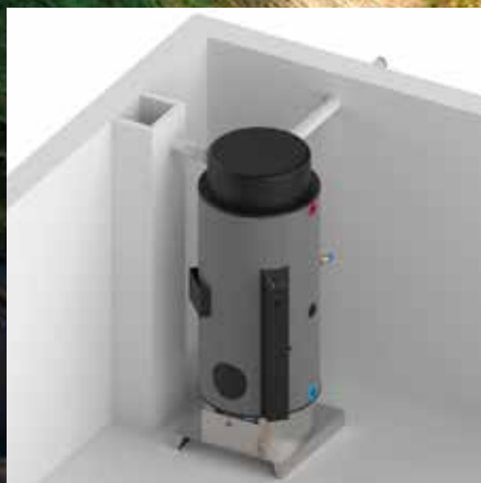
Inlet Air and Existing Flue
